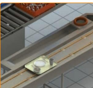
Wet trough, width 220mm 'conveyor sediment's'
