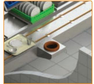
Removable sorting block equipped with a waste hole for frontal orting
