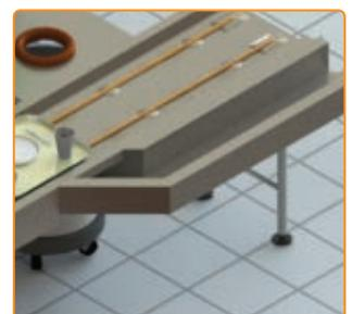
Wet trough of a 500 mm length for passing under the conveyor
